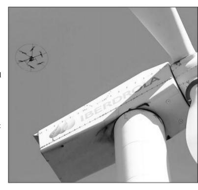
The Aracnocóptero Eoló performs the same functions, but more quickly, and is also capable of detecting precisely any type of erosion or damage, which is why it stands out. It also allows them to act early and avoid more severe damages.
